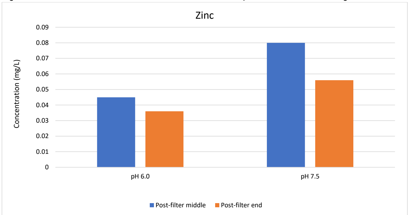
Figure 4: Zinc concentration after filtration. Zinc concentration prior to filtration was 20 mg/L.
