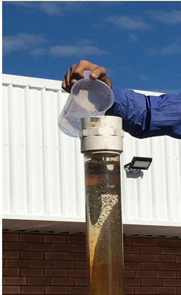
Figure 1: Filtration of the test water and filling of test filtration unit.
